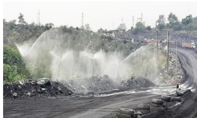
Rotating Fixed Sprinklers near Quarry Bottom Stock
